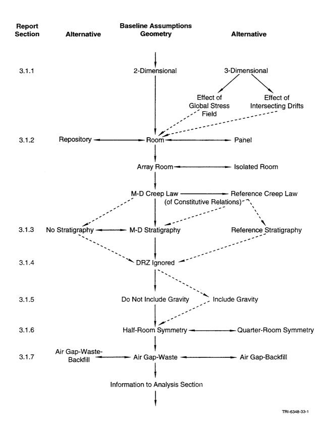
Figure 1. Repository geometry models and assumptions. The symbol ↔ indicates that the alternative can be substituted for the baseline assumption. Dashed lines indicate unlikely path options.
