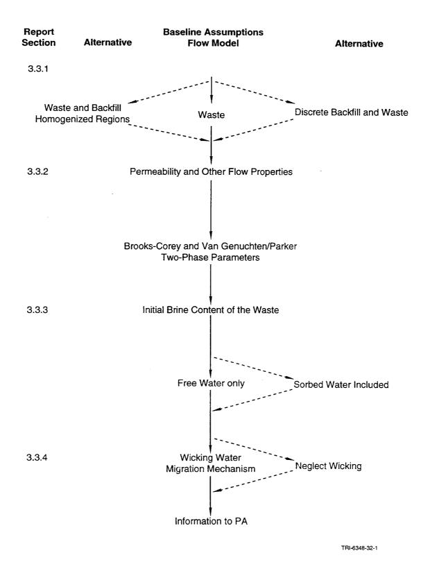
Figure 3. Waste and backfill flow models and assumptions. Dashed lines indicate unlikely path options.
